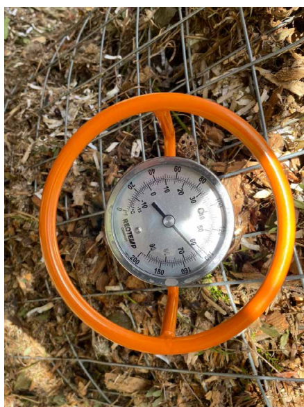
Figure 7. Compost thermometers that are purpose designed to keep a close eye on temperatures of the compost pile [Photos: Mary Retallack].
